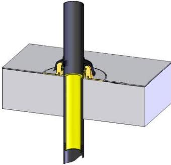
Postpone the rain deflector from above over the PE-pipe up to the base plate.
