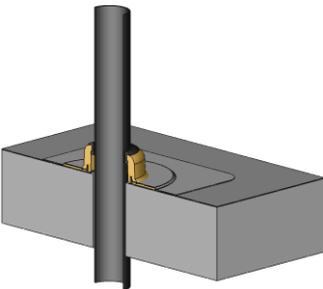
Reap the PE-pipe from the outside with lubricate and push it through the sealing ring of the installed base plate to the desired height.
