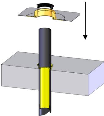
Insert the sealing ring into the SitaVent pipe system base plate. Reap the installed PE-pipe from the outside as well as the sealing ring from the inside with lubricant and postpone it from above over the connection pipe. Fix the base plate mechanically with the roof construction.
