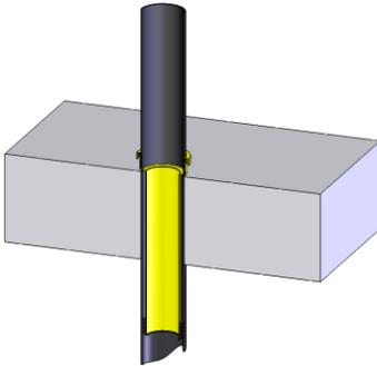
Insert the SitaVent pipe system PE-pipe into the coupler of the Sita Redevelopment adapter by using lubricate.
