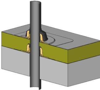
Slide the rain deflector from the top over the PE-pipe up to the base plate.
