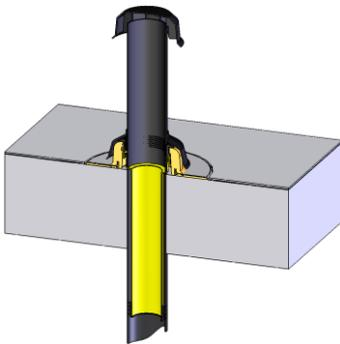
During the insertion of the rain cover or the protective grating, the fixing ring needs to be put on the installed PE-pipe and postpone the rain cover without lubricate or the protective grating with lubricant.
