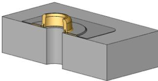
Place the SitaVent pipe system base plate centered over the roof opening of the roof construction and fix it mechanically.
