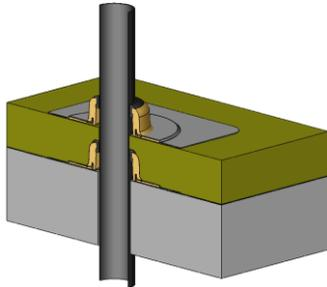
Insert the sealing ring into the base plate. Reap the built-in PE-pipe from the outside and the sealing ring from the inside with lubricant and slide the base plate from the top over the connecting pipe. Fix the base plate mechanically to the roof construction.
