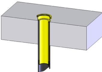
Reap the inside of the to be renovated pipe with lubricate and insert the SitaRedevelopment adapter from above.
