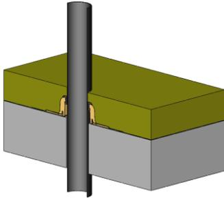
Cut the negative of the base plate into the thermal insulation and mount the thermal insulation.
