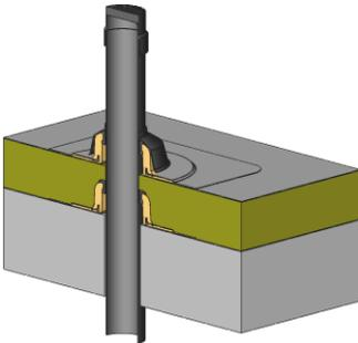
When using the rain cover or the protective grating, set the fixing ring on the installed PE-pipe and postpone the rain cover without lubricant or the protective grating with lubricant.
