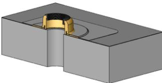
Glue or weld the roof track with the connection sleeve of the base plate.
