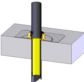
Weld or glue the roof sealing with the base plate connection sleeve.
