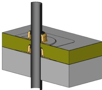
Glue or weld the roof sealing with the base plate connection sleeve.
